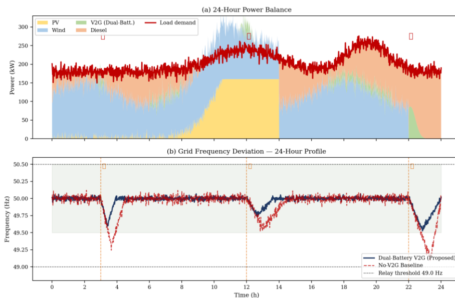
Fig. 2. 24-hour simulation results: (a) power balance showing PV, wind, V2G, and diesel contributions versus load demand; (b) grid frequency deviation profile for the proposed dual-battery V2G versus no-V2G baseline. Event markers ①②③ indicate disturbance injection instants.
