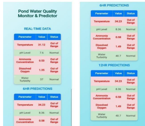
Fig. 4 Web dashboard interface showing real-time water quality and predictions.
