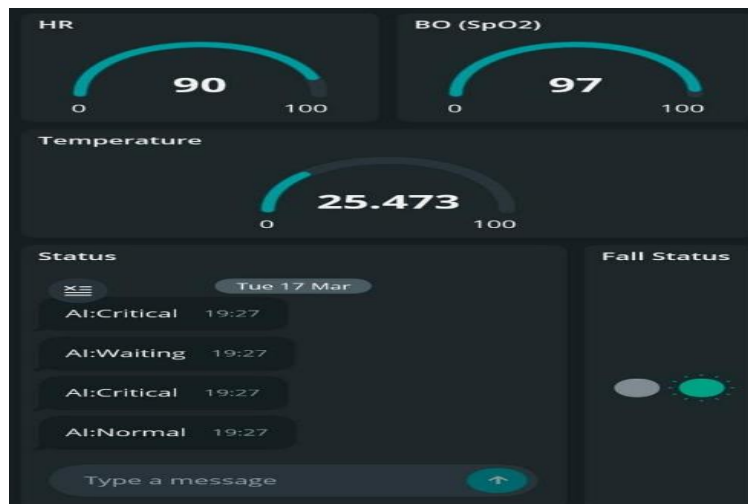
Figure 4 Real-Time Vital Monitoring System with Normal Fall Status Indication
