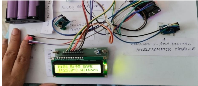
Figure 3 Normal Condition Display of the Monitoring System
