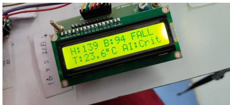
Figure 6 Health Monitoring Dashboard (Critical Alert State)
