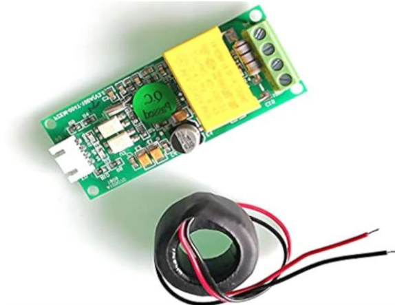
Fig 3.1: CT Sensor and PZEM-004T Energy Meter Module
