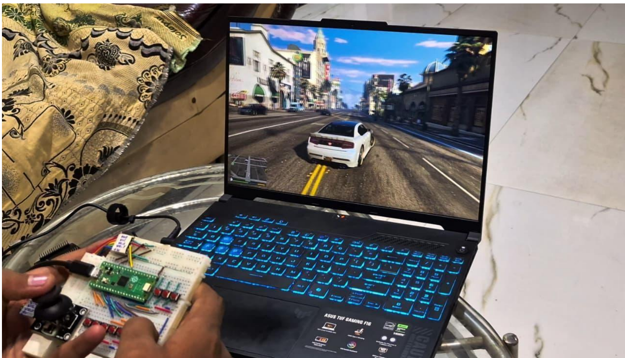
Fig. 5. Live gaming demonstration: controller (Version 3 breadboard prototype) used to play Grand Theft Auto V on Windows 11 (ASUS TUF Gaming F16). Joystick provides camera/character/mouse control; buttons map to game actions.
