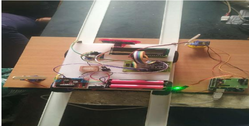
Fig 5: Working Model of Railway Track Crack Detection and Automatic Gate Control System
