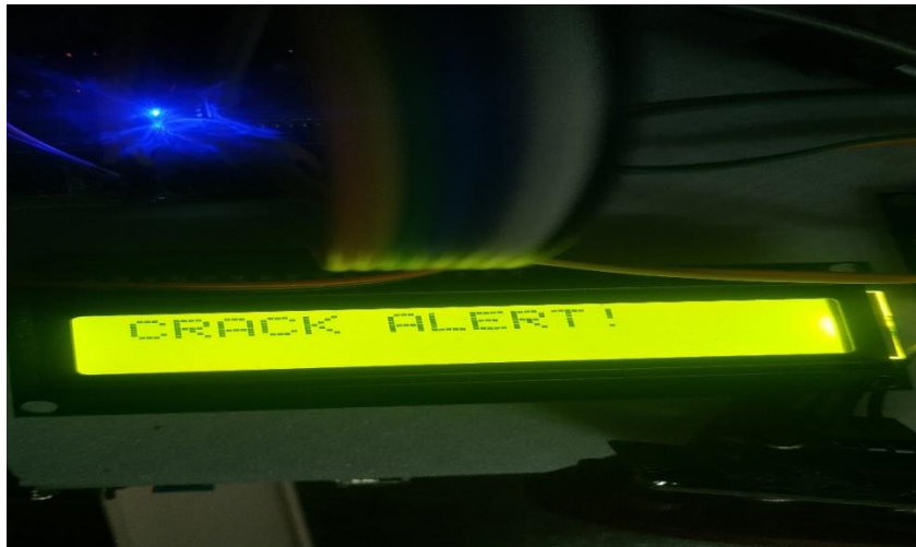
Fig 6: LCD Display Showing Crack Detection Alert
