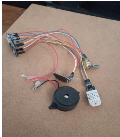
FIG5: IOT Based Temperature and Pressure Monitoring System
