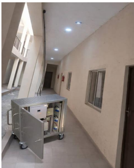
Figure 6: The developed energy storage system, powering school office
