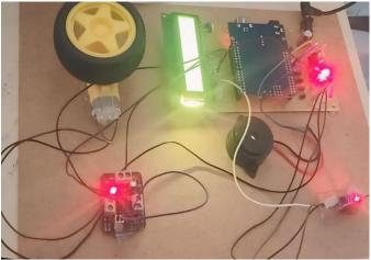
A microcontroller-based automatic engine locking system for drunken drivers aims to prevent accidents by detecting alcohol levels in the driver's breath and automatically locking the engine
