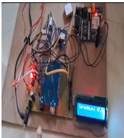
Figure 3: Smart garbage monitoring system when the garbage is filled it send a sms and location
