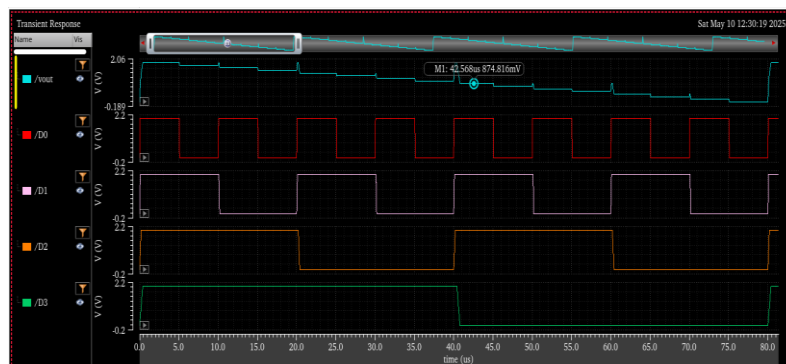
Fig. 7: Transient Analysis of 4 bit R-2R DAC
