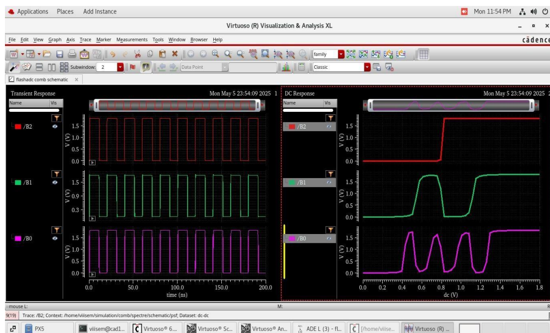
Figure 12 TIQ Flash ADC's Output
