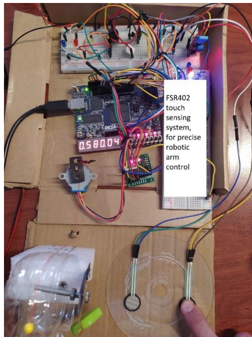
Figure 5c: FSR 402 touch-sensing system for precise robotic arm control, operating.
