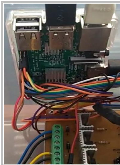
Figure 5. Raspberry Pi Model 3B showing its connections to external interface circuit and some attached peripherals
