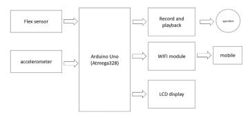
Accelerometer sensor measures the linear movements of hand in X-axis, Y-axis, Z-axis and outputs different values of X, Y, Z corresponding to the movement in X-axis, Y-axis, Z-axis.
