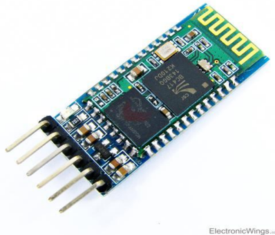
Figure 5: Bluetooth Module (HC-05)
