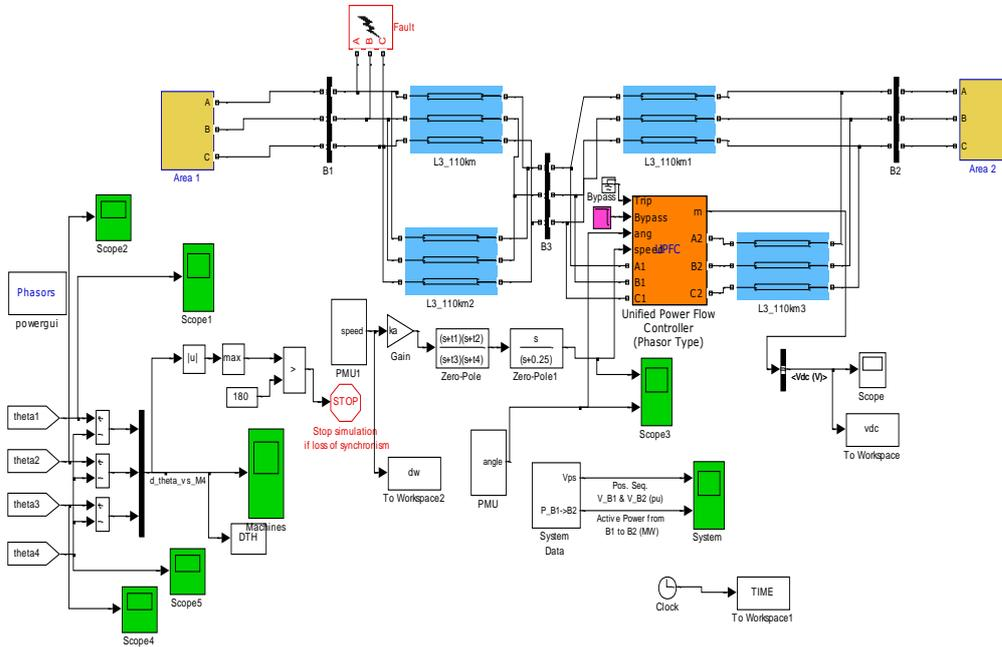
Fig.4. Simulation diagram for both GA based PSS and PSO based PSS with UPFC.
