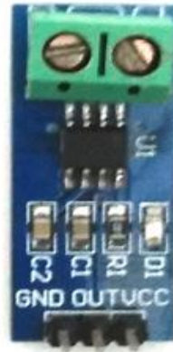
Fig 5: ACS712 Current sensor
