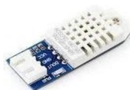
Fig 5: DHT22-temperature and humidity sensor
