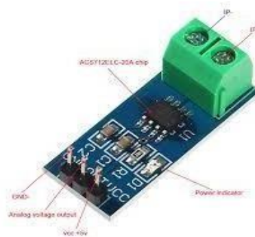
Fig 4: ACS712-current sensor
