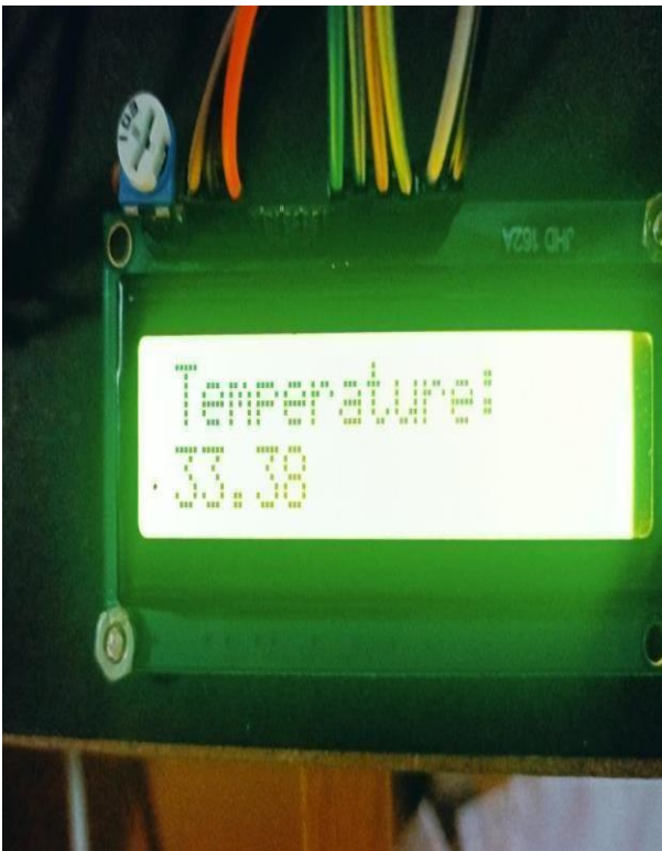
Fig.6: The body temperature shown in LCD display
