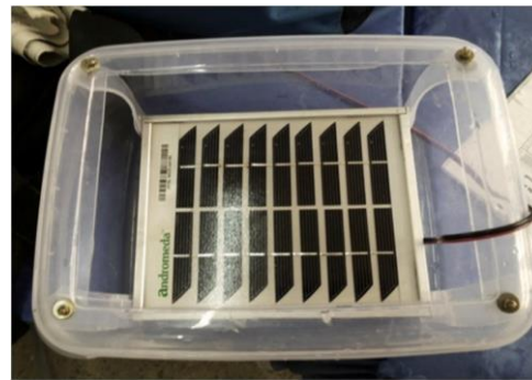
Fig. 7 Illustrates liquid immersion refrigeration.
