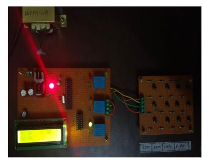
In this module, we employed an underground cable fault detector. Initially, instead of cables, resistors were utilized. The initial readings displayed R=0, Y=0, B=0 kilometers.
