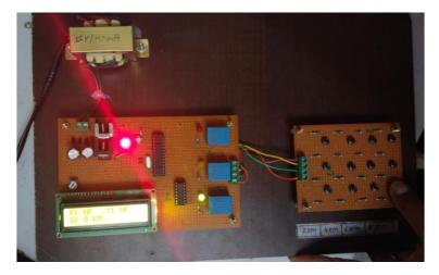
To induce a fault in the B-phase at a distance of 8 kilometers, simply ground the switch. This sets B=8 kilometers. Consequently, the respective B-phase relay deactivates, as indicated by the LED.
