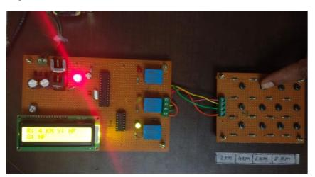
To induce a fault in the "R" phase at a distance of 4 kilometers, simply shift the switch towards the ground. Grounding this switch signifies that R=4 kilometers. Consequently, the corresponding R-phase relay deactivates, as indicated by the LED.
