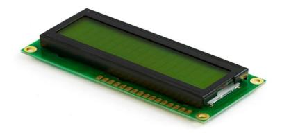
LCD (Fluid Gem Show) screen is an electronic show module and discover a wide extend of applications. A 16x2 LCD show is exceptionally fundamental module and is exceptionally commonly utilized in different gadgets and circuits. These modules are favored over seven fragments and other multi section LEDs.
