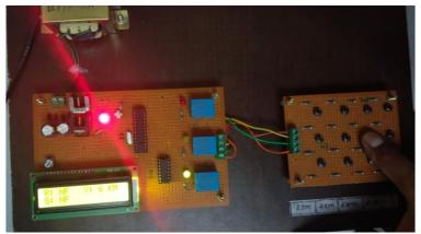
To induce a fault in the Y-phase at a distance of 6 kilometers, simply ground the switch. This action sets Y=20 kilometers. Subsequently, the respective Y-phase relay deactivates, as indicated by the LED.
