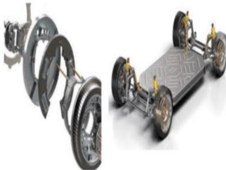
Fig. 1 Ecosystem – Protean Electric: In-wheel/Hub Motors
