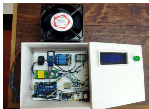
3(b). Internal Circuit Connected to Fan Load
