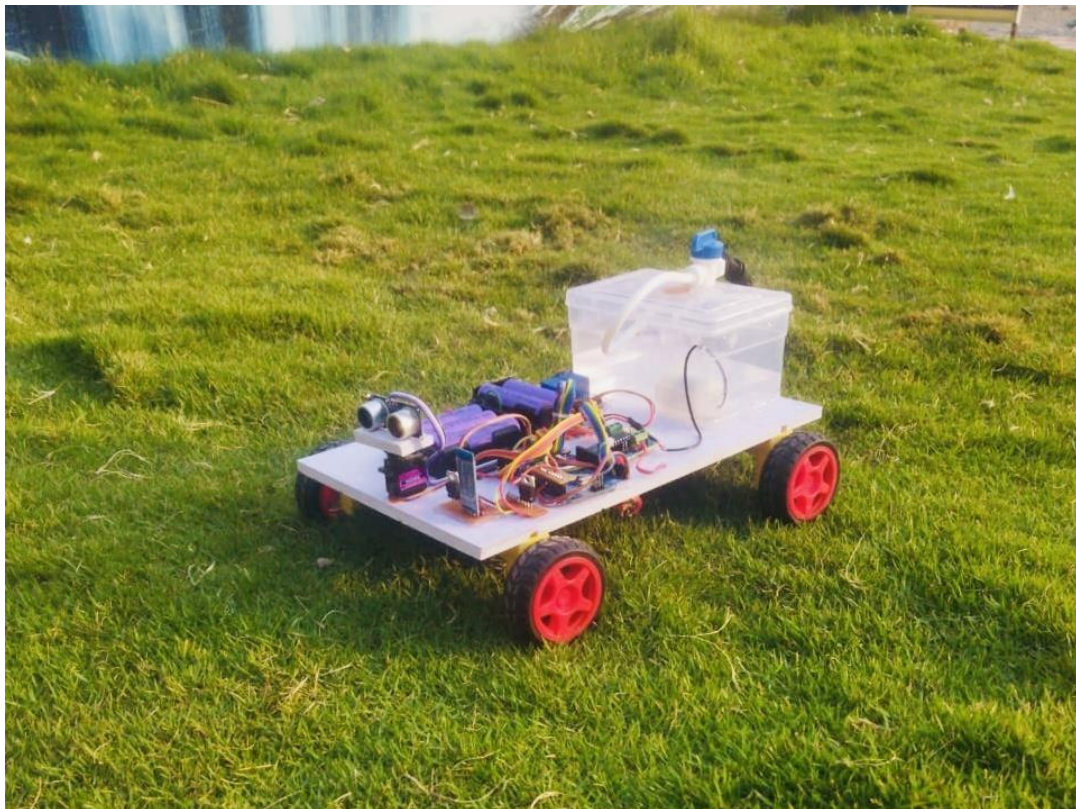
Fig 3: The Machine Is Moving On The Right Side Due To Obstacle Detection On The Left Side.
