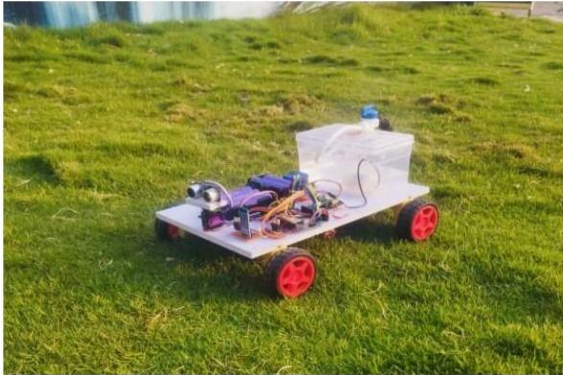
Fig 4: Model of “Design and operation of agriculture Based pesticide spraying and Grass Cutting Robot”
