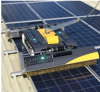
Fig. 4: Mechanical cleaning of solar PV panels [12].
