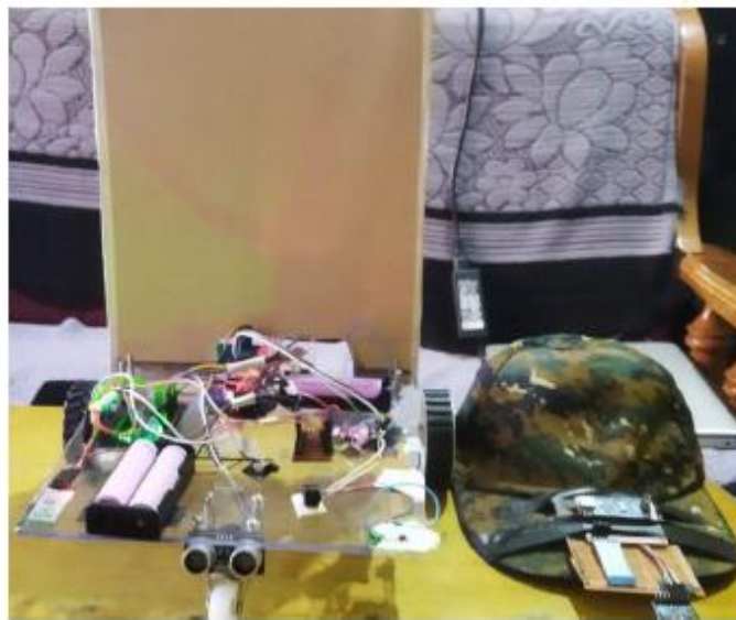
Fig 6: Prototype of wheelchair controlled by Head Motion
