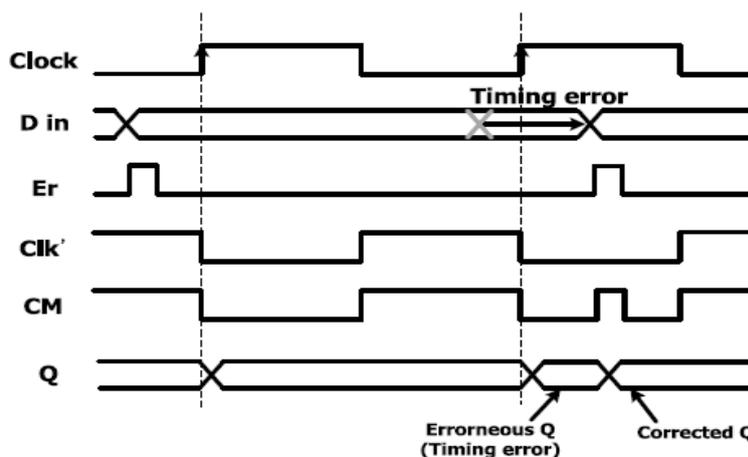
**Fig. 2. Operation of the proposed system when a timing error occurs.**
