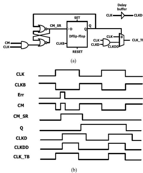
Fig. 4. Time-borrowing technique. (a) Time-borrowing circuit structure. (b) Operation of the time-borrowing system.
