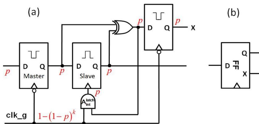
Fig.6 Enhanced AGFF with XOR output used for LACG.
