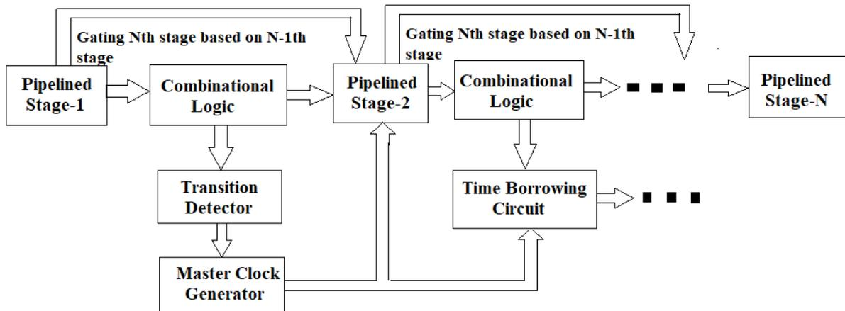
Fig. 3. Proposed Timing-error-tolerant circuit.
