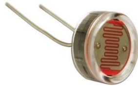
Fig.6 Light Dependent Resistor [27]
