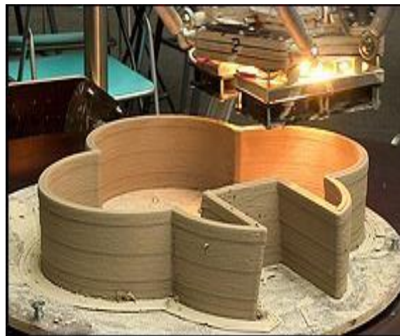
A WASP Big Delta 3D printing in clay
