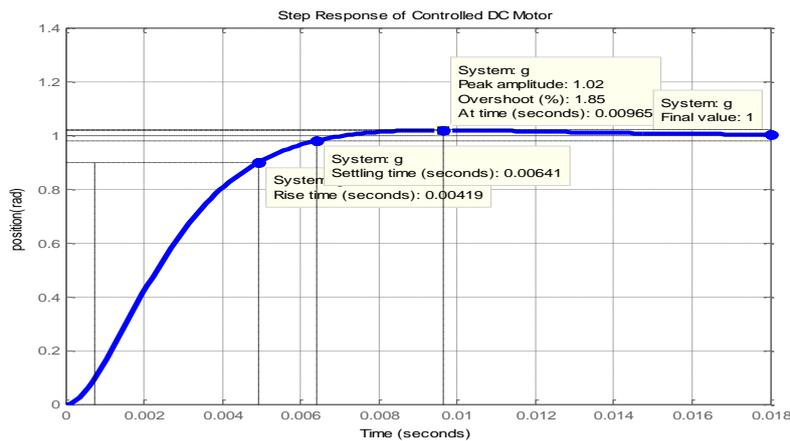
Figure 7 Step response of controlled DC motor.
