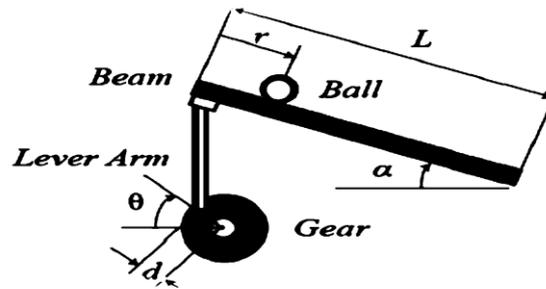
Figure 3: Ball and beam model [11,12]
