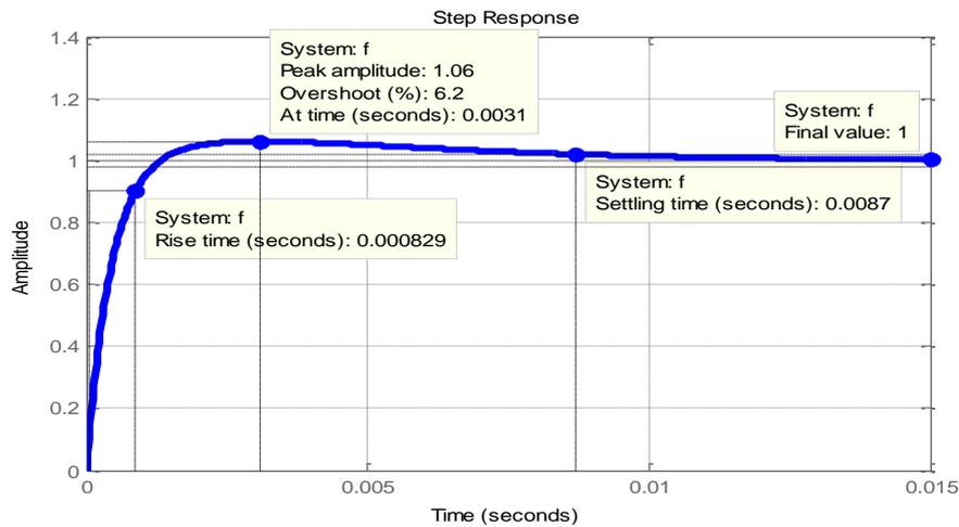
Figure 12: Step Response of the Controlled System
