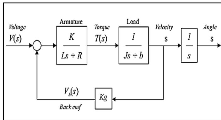
Figure 2: A block diagram of the DC motor[10]
