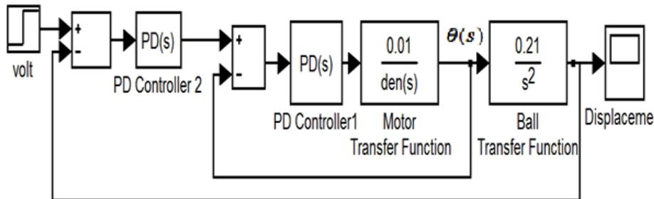
Figure 11: BBS with PD controllers
