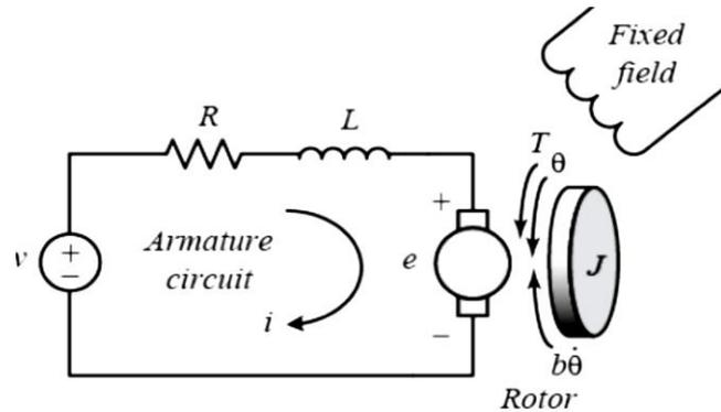
Figure 1: Equivalent circuit of a DC motor[9]
