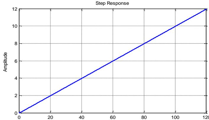
Figure 5: Open-loop response of the uncontrolled DC motor
