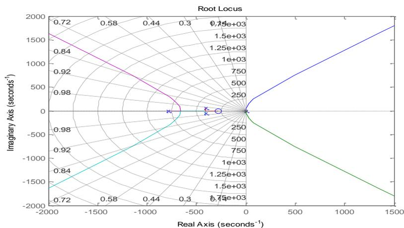
Figure 10: Root locus of the uncontrolled ball and motor system
