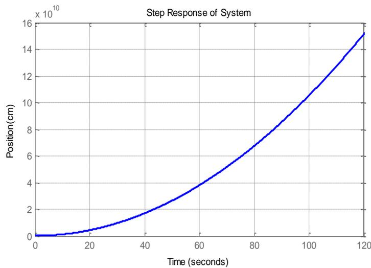
Figure 9: Step response of an uncontrolled ball and motor system
