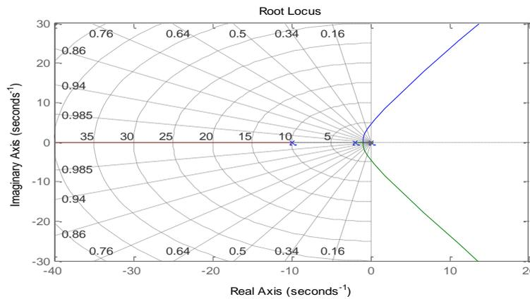
Figure 6: Root locus of the uncontrolled DC motor
