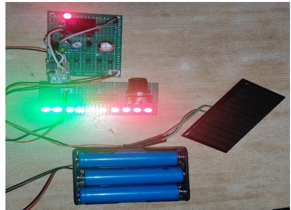
FIG. 10 100% BATTERY LEVEL AND IT IS IN FULLY CHARGED STATUS
