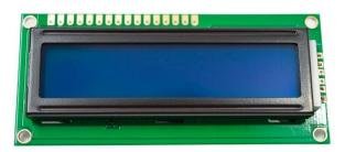
The 1602A LED display, also called as 16x2 alphanumeric display, is a commonly used output device that allows for the visual display of characters, numbers, and symbols. It consists of 16 columns and 2 rows of alphanumeric characters, providing a total of 32 displayable characters.
