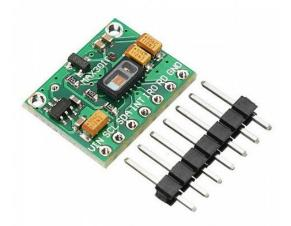
Place The MAX30100 is a versatile sensor module that combines two primary functionalities: a pulse oximeter and a heart rate sensor. It uses optical sensing techniques to measure heart rate and blood oxygen saturation (SpO2) non-invasively. Here's a sharp and precise description of the MAX30100 heartbeat sensor:
