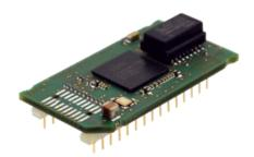
I2C modules, also known as I2C interfaces or I2C controllers, are electronic components that facilitate communication between devices using the I2C protocol.
