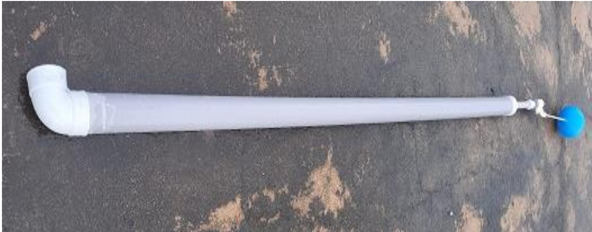
Fig 9 Automatic float valve fitted in tank
