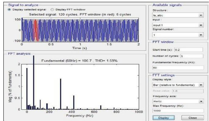
The utility power source current after the harmonic compensation is illustrated in Fig. 7. The THD (Total Harmonic Distortion) is also computed in load current as well as in supply current. The THD is 19.19% before harmonic compensation in load current and 1.59% in supply current after harmonic current compensation that is within the limit of the harmonic standard of IEEE 519.
