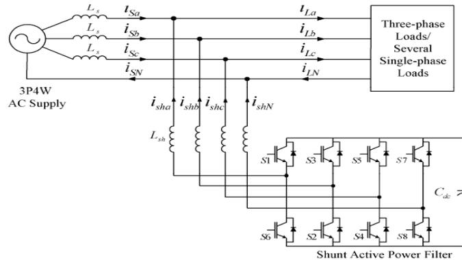
Fig.1 Four-leg(4L) based 3P4W shunt active power filter topology.
