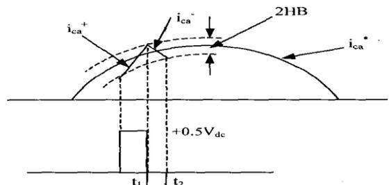
$$HB = \left\{ \frac{0.125V_{DC}}{f_c L} \left[ 1 - \frac{4L^2}{V_{DC}^2} \left( \frac{v_s}{L} + m \right)^2 \right] \right\} \tag{8}$$
