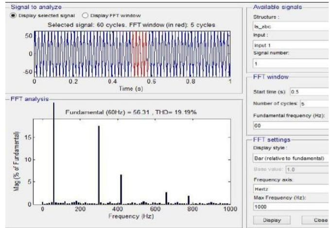
**Fig. 7:**FFT Analysis of 4LEG TOPOLOGY
