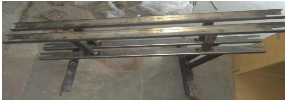
Fig. C channels assembled on each other on square tubes
