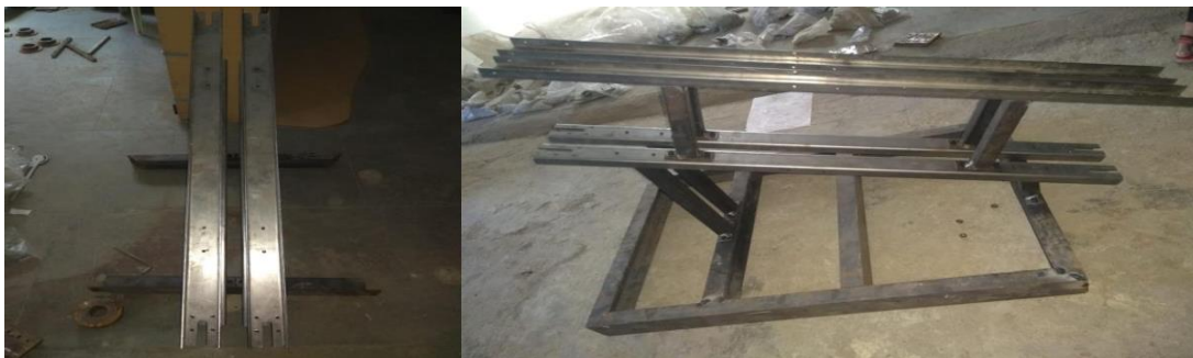
Fig.7.2 c channel assembled on the main frame
