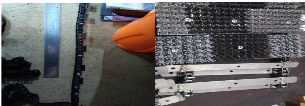
Fig. chain with attachments and support plates for conveyor material or mat
