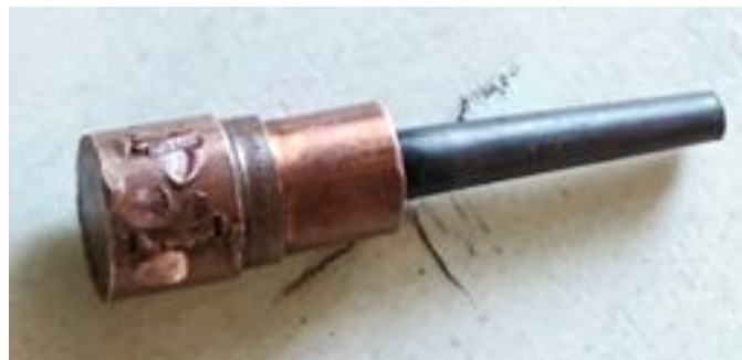
Figure 1: Copper tool electrode utilized for experimentation
