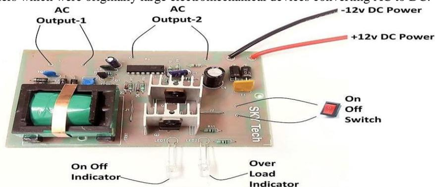
A power inverter, inverter or invertor is a power electronic device or circuitry that changes direct current (DC) to alternating current (AC). The resulting AC frequency obtained depends on the particular device employed. Inverters do the opposite of rectifiers which were originally large electromechanical devices converting AC to DC.
