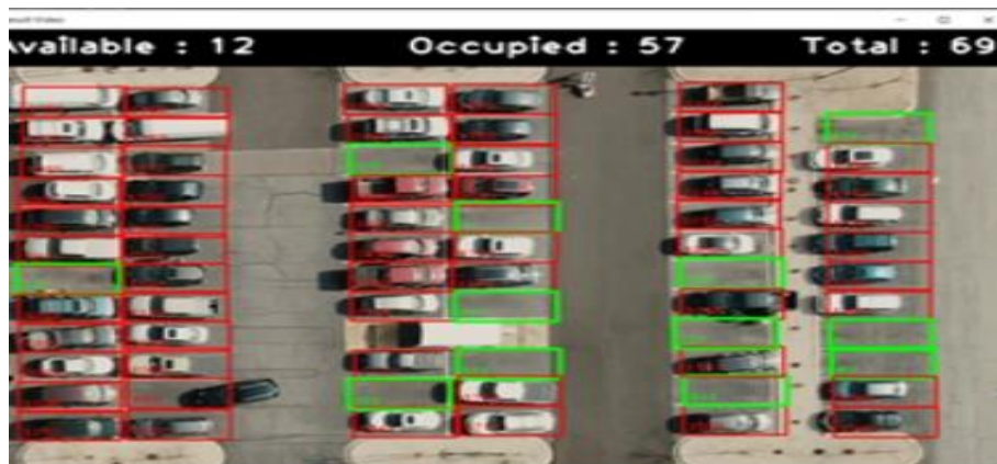
Fig.11 Vehicle Detection and Occupancy Output
