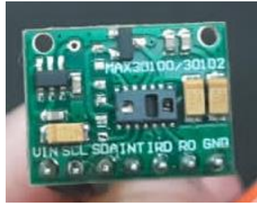
Fig. 4. SpO2 And BPM Sensor
