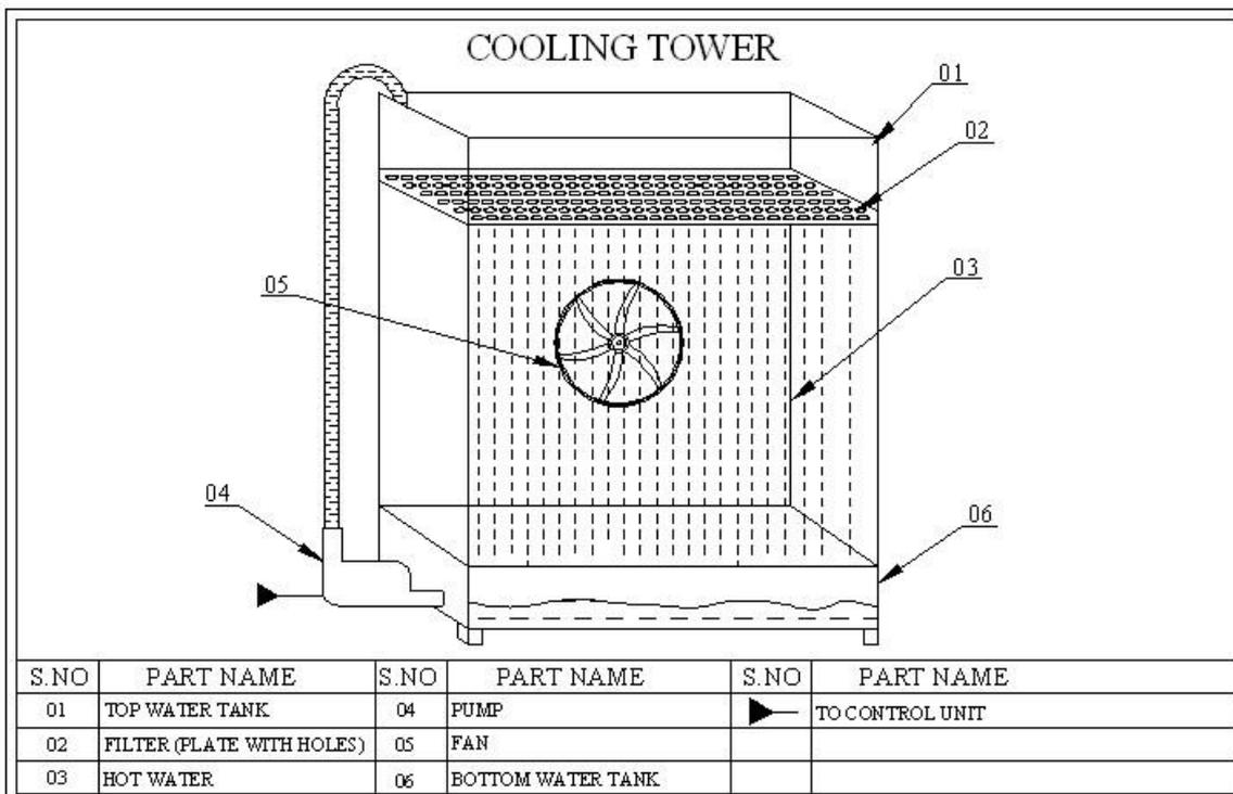
**DRAWING FOR TEMPERATURE CONTROLLER WITH COOLING SYSTEM**
