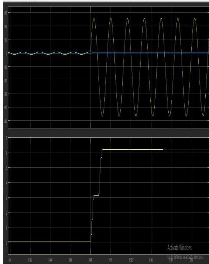
Fig. 6 Waveforms of DC reactors and AC reactors current at single-phase (phase a) to ground accident.
