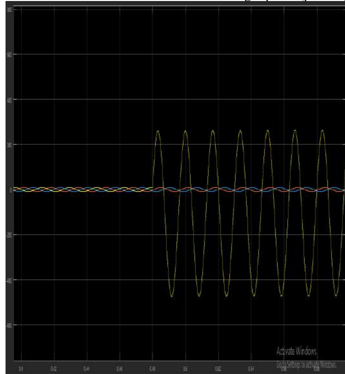
Fig. 9 Waveforms of load current and voltage drop upon transformer primary windings at single-phase (phase a) to ground accident.
