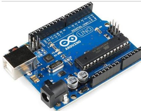
The Arduino Uno can be powered using either a USB connection or an external power supply. A battery or an AC to DC adapter are the most common external power supplies. The Arduino Uno can be connected to the adapter by inserting it into the Arduino board's power port. Similarly, the battery leads can be connected to the POWER connector's Vin and GND pins. The recommended voltage range is 7 volts to 1 volt.
