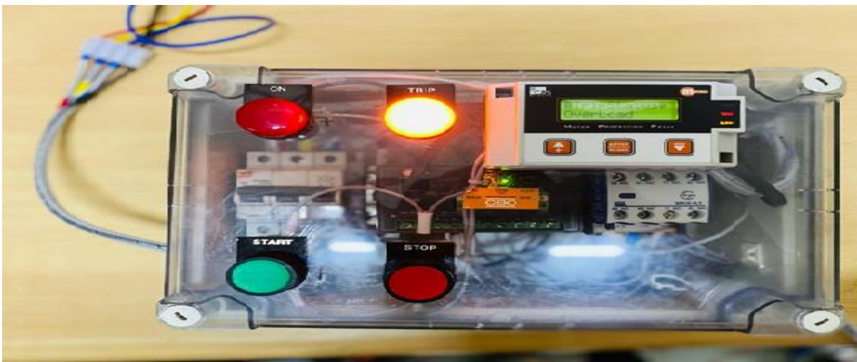
Fig. 6 Overload tripping status (IDMT Characteristic)
