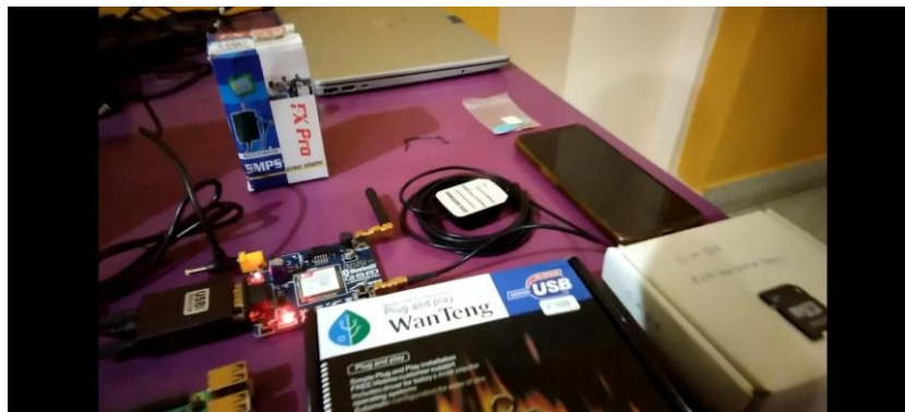
Figure(3): Demonstration Of User's Acknowledgment, Switching Action (ON/OFF) Controlled By GPRS, GPS Modules.
