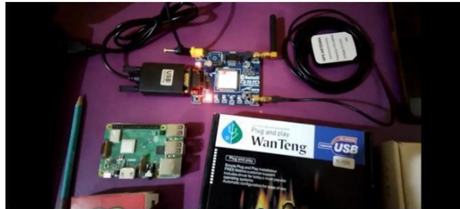
Figure (3) Simulation of GPS, GPRS using GSM module to locate the vehicle
