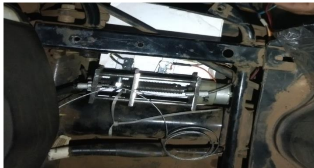
Fig 4.2 Practical implementation of Speed Governing Mechanism on two wheeler vehicle
