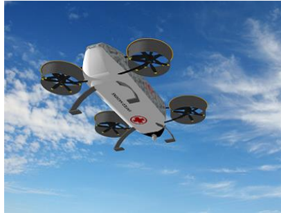
Fig2: A ducted-propeller UAV in flight [Source: https://www.amatek.com/case-studies.html ]
