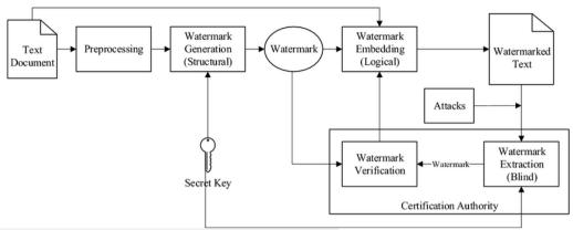
(Digital text watermarking (embedding and extraction) architecture.)
