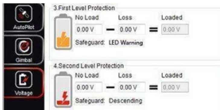
Fig. 7 Drone Battery Protection Level
